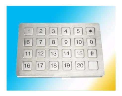
24 keys compact format IP55 dynamic vandal proof Stainless Steel encryption PINPAD with industrial encryption electronics controller supporting DES/TDES shieded & protected by stainless steel housing, industrial PCB with carbon-on-gold key switch technology with long stroke (2.0mm) with extremely good tactile feeling for fast and accurate data input without any noise, top stainless steel plate with threaded bolts under top stainless steel plate for top panel mounting solution
